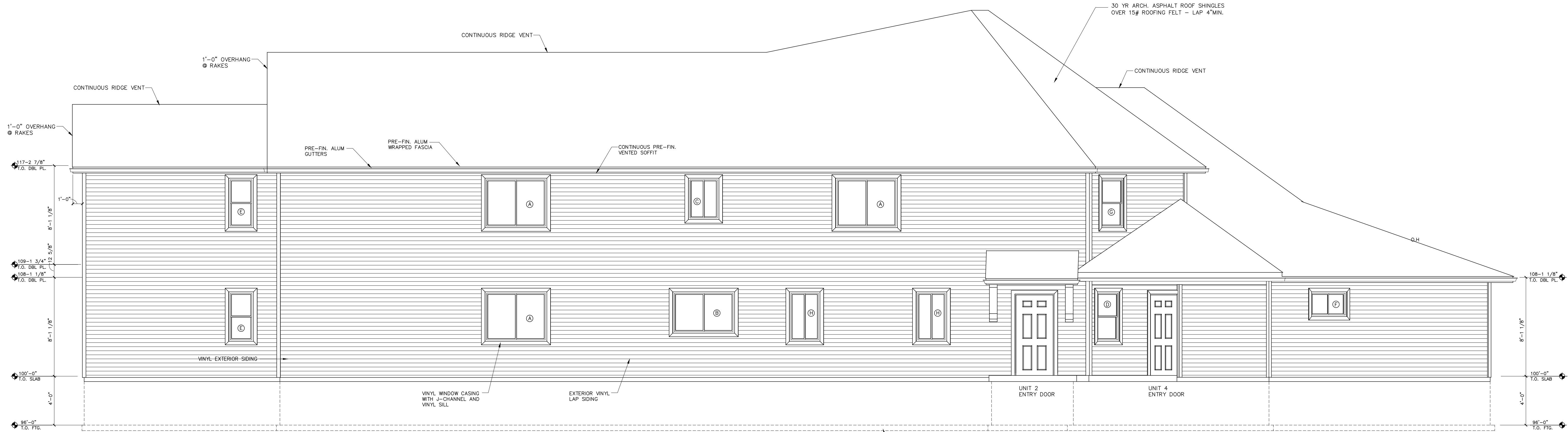
1 RIGHT SIDE ELEVATION - SOUTHEAST 1/4" = 1'-0"
